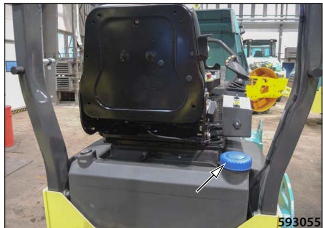
Remove the drain plug of the water tank.
