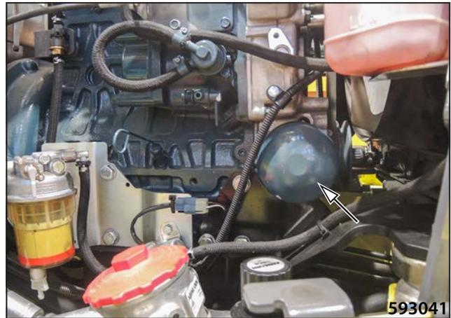
Lubricate the gasket with oil.
