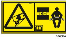
Fasten the safety belt before the machine starts moving.
