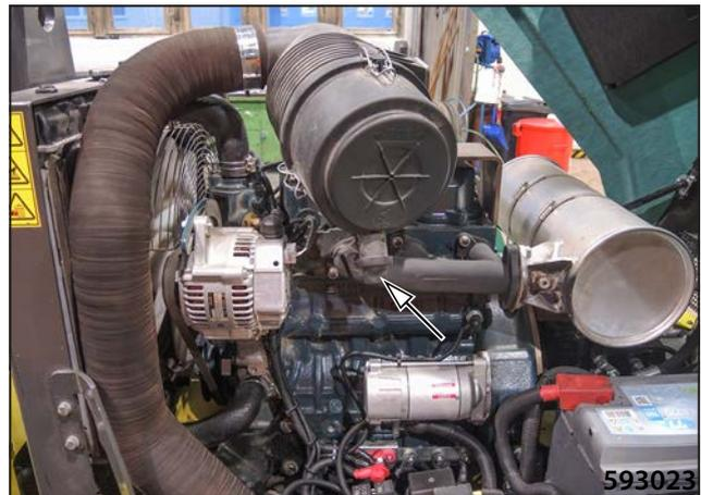
Check connections and the piping for leakage and the engine inlet opening on the bonnet for clogging (e.g. by leaves).
