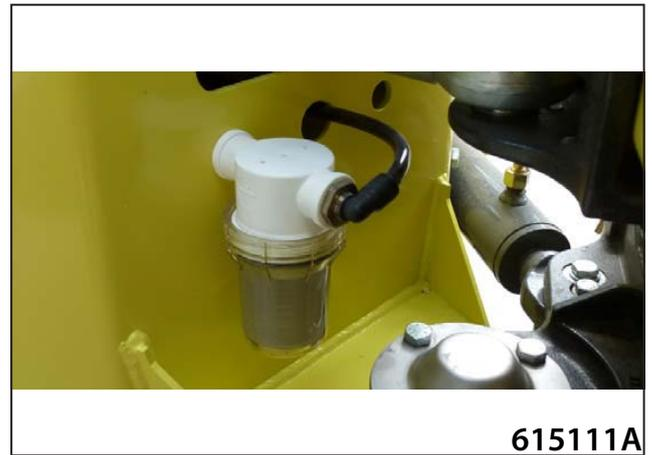
Remove and clean the sprinkler strainers.
