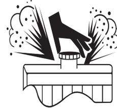
Avoid inhaling airborne particles or spray from coolant. If the substances make contact with skin or eyes that are not protected by personal protection gear, immediately wash the skin and eye with flowing water for 20 minutes or longer.
