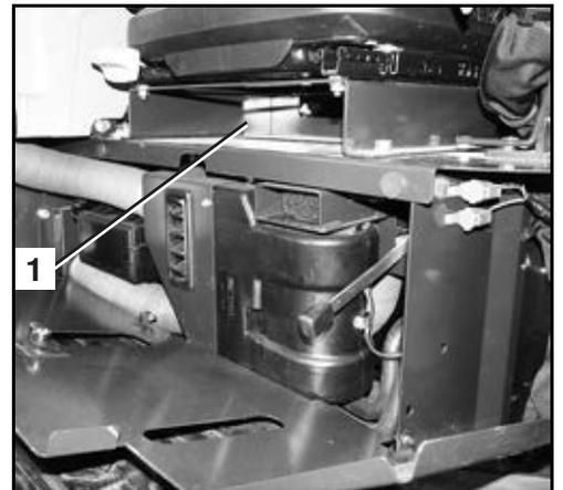
The grease gun must be stowed in the storage location (1) behind the left service cover on the swivel frame.
