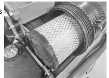
1. Squeeze the rubber vent on the filter housing cover to drain water and dirt from the filter.
