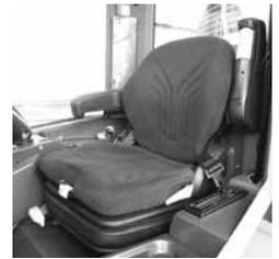
The seat is equipped with heater. Heater switch is located on the back rest on the left. Below it is located the lumbar support adjustment.
