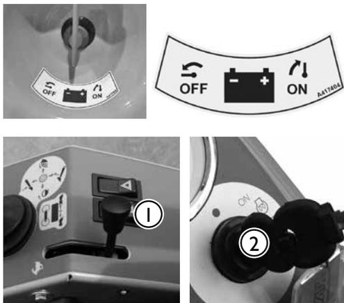
1. Turn the battery disconnect switch to ON
