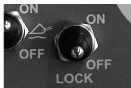
**LOCK OFF:** In this mode, the hydraulic oil flows in series from motor to motor. The wheels will roll more freely and the loader leaves less tire marks on soft surfaces.
