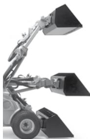
NOTE: Self leveling is disabled when the boom floating is switched on.
