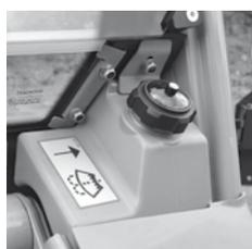
Windscreen washer tank and filler cap on machines with cab LX and DLX are located outside the cab, in front of the windscreen on the left.
