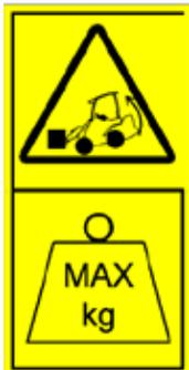
**Overload will cause the loader to tip forward.** Always pay attention to safe operating conditions whenever lifting loads or handling heavy attachments.
