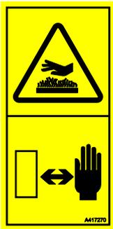
**Risk of burns - Hot parts.** Allow engine to cool before accessing the engine. Engine and exhaust parts may be extremely hot after use.
