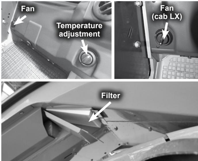
Heater temperature adjustment on cab LX/DLX is located in the footwell left. On cab LX also the fan speed switch is located in the footwell. On cab DLX fan speed switch is located in the control panel up right.
