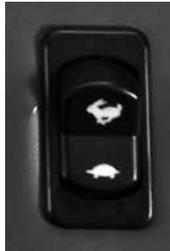
Higher speed range is intended for longer travels where high pulling force is not necessary.
