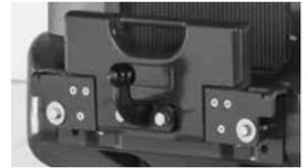
Max. allowed vertical load of the trailer coupling is 6900 N, max. towing load is 6000 N.
