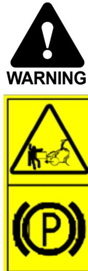
**Risk of being crushed by moving loader - Engage parking brake before working near the loader.** Follow safe stopping procedure to prevent all movements of the loader. Avoid leaving the loader parked on hill. If necessary to park on hill, use chocks or other additional means to prevent the loader from moving.
