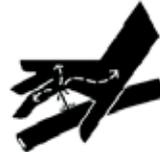
**Never handle hydraulic components if hydraulic system is pressurized - Risk of injection of hydraulic oil through skin.**
