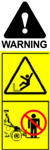
**Falling of persons - Risk of crushing.** Never use the loader or its attachments to lift persons or as any kind of work platform even temporarily. Never climb on the loader or on the attachment. Seating capacity: one person only, regardless of attachment.
