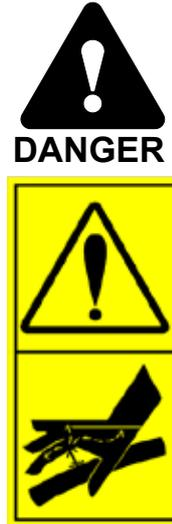
**Hydraulic pressure - Risk of injury.** Escaping hydraulic fluid under pressure has sufficient force to penetrate skin, causing serious personal injury. Never use hands to search for possible leaks in hydraulic systems - use a piece of cardboard instead. Release residual hydraulic pressure before disconnecting any fitting and before any service operation. See a physician immediately if hydraulic fluid penetrates skin, serious injury can result quickly.
