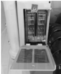
The main fuse box on loaders with cab LX/DLX is located outside the cab, on the right side below the windscreen under a metal cover.
