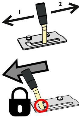
You can use either this lever or the buttons of the electric joystick (optional equipment) to operate the the attachment. Release the lever to its neutral position when you stop using the loader.
