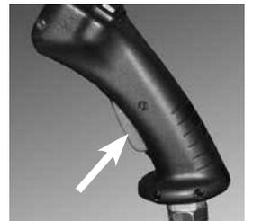
**X-lock OFF:** The anti slip valve equalizes the oil flow between the left and right hydraulic motors, but some oil will pass between the left and right side of the loader through the open X-lock valve.
