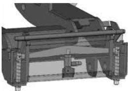
The hydraulic attachment coupling plate enables connecting and disconnecting of the attachment from the driver's seat. There is a hydraulic cylinder on the attachment coupling plate which moves the locking pins up and down. The electro-hydraulic system works also when the engine is not running, as long as the ignition switch is in "ON" position (current on). Control switch is located at the control panel on the right (see page 24).
