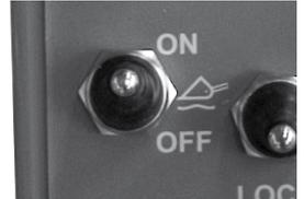
NOTE: The switch is installed on the dashboard, also in cases the boom floating option is not installed on the loader. The presence of the switch does not mean the boom floating or Smooth drive options are fitted.
