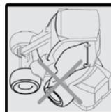
Do not drive with the cab door open, nor turn the steering wheel when the cab door is open. The door may break upon contact with wheels.
