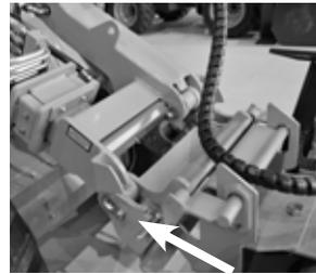
The red service support of the boom lift cylinder is located at the tip of the boom, behind the attachment coupling plate. Make sure that the boom stays up during maintenance operations by attaching the service support on the lift cylinder piston rod. Secure the service support by locking it on the piston rod with the long screw that is on the support.
