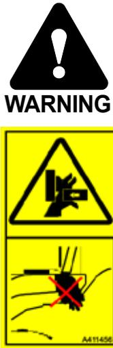
**Pinching points** - Avoid pinching between loader frame itself and between loader and walls - Keep all body parts within the safety frame. Movements of the articulated frame creates pinching hazards. Keep your head, hands, and feet inside the loader. Be especially careful while you drive near walls and trees. Keep your hands on steering wheel and joystick.
