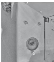
On machines with cab L the tank is located behind the front left wheel and the filler opening is on the footboard.
