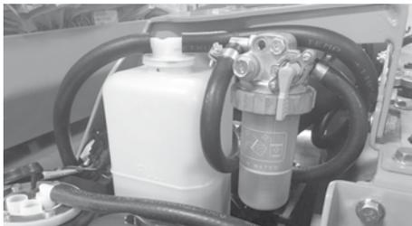
Never open the pressurized radiator, when the engine is warm. Hot coolant may burst out causing serious burns. Allow the engine to cool completely before opening.
