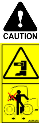
**Avoid pinching hazard for legs - Do not turn the steering wheel while standing near the loader.** Turning the articulated frame creates a pinching hazard to a person standing near the tyres of the loader. Never grab the steering wheel while entering or leaving the driver's seat to avoid turning of the frame. Stop the loader if other persons get close to it. Check that tyres that are larger than standard tyres leave enough space between the tyres for safe use.
