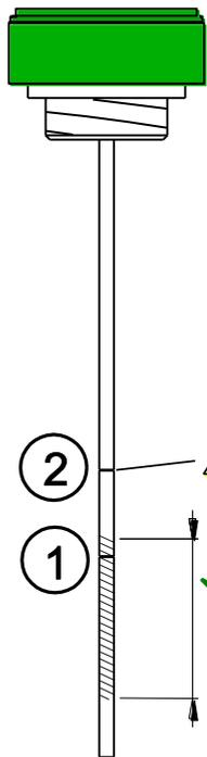
1 Target marker. Fill to this mark when hydraulic system is cold. The area highlighted in the adjacent figure shows approximately the acceptable level.
