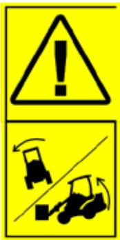
**Risk of tipping over - Always keep loads close to the ground.** The stability and the load handling capacity of the loader are significantly reduced on inclined terrains and Maximum lifting capacity can be achieved only on firm, level ground. On horizontally tilted terrain the load must be kept close to the ground and must never be lifted high.
