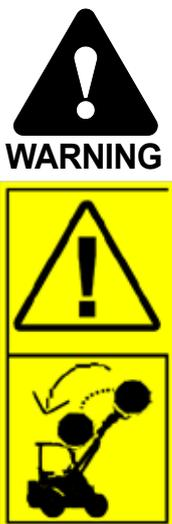
**Risk of falling objects - Make sure load is securely on the attachment.** Never tilt an attachment back when it is lifted high. Make sure the loader is equipped with ROPS and FOPS structures that are in good condition and do not have visible damage. Make sure the attachment is properly locked.
